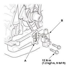
3. Remove the pin from the cam chain auto-tensioner.
