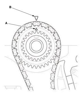
Set the crankshaft to top dead center (TDC). Align the TDC mark (A) on the crankshaft sprocket with the pointer (B) on the engine block.
