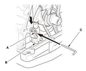
3. Rotate the crankshaft counterclockwise to align the holes on the lock (A) and the cam chain auto-tensioner (B), then insert a 1.2 mm (3/64 in) diameter pin (C) into the holes. Turn the crankshaft clockwise to secure the pin.
