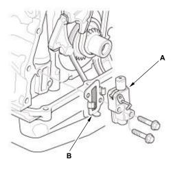
4. Remove the cam chain auto-tensioner (A) and the cam chain auto-tensioner filter (B).
