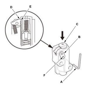
Compress the cam chain auto-tensioner when replacing the cam chain. Remove the pin (A) from the cam chain auto-tensioner that was installed during removal. Turn the plate (B) counterclockwise, to release the lock, then press the rod (C), and set the first cam (D) to the first edge of the rack (E). Insert the 1.2 mm (3/64 in) diameter pin back into the holes (F).
