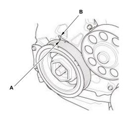
Turn the crankshaft so its white mark (A) lines up with the pointer (B).
