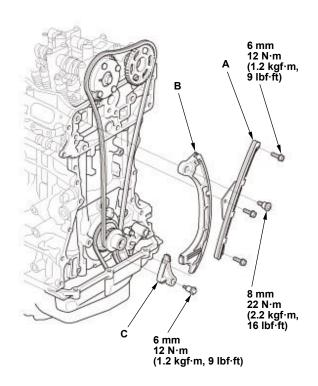
Install cam chain guide A, the cam chain tensioner arm (B), and the cam chain tensioner sub arm (C).
