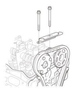
Remove cam chain guide B.
