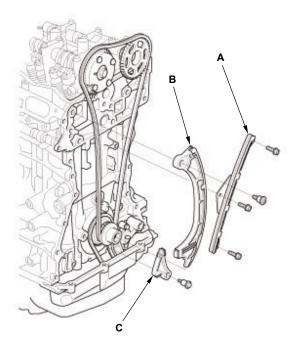
Remove cam chain guide A, the cam chain tensioner arm (B), and the cam chain tensioner sub arm (C).
