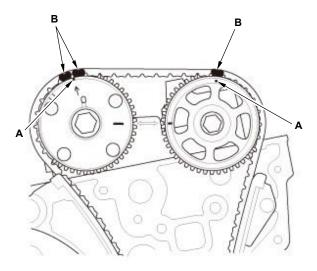
2. Install the cam chain on the VTC actuator and the exhaust camshaft sprocket with the punch marks (A) aligned with the center of the two colored link plates (B).
