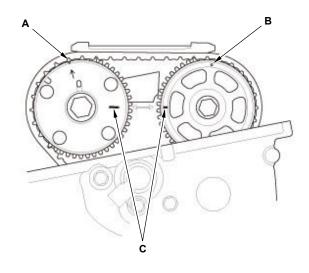
Set the No. 1 piston at top dead center (TDC). The punch mark (A) on the VTC actuator and the punch mark (B) on the exhaust camshaft sprocket should be at the top. Align the TDC marks (C) on the VTC actuator and the exhaust camshaft sprocket.
