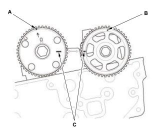
Set the camshafts to TDC. The punch mark (A) on the VTC actuator and the punch mark (B) on the exhaust camshaft sprocket should be at the top. Align the TDC marks (C) on the VTC actuator and the exhaust camshaft sprocket.
