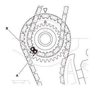
1. Install the cam chain on the crankshaft sprocket with the colored link plate (A) aligned with the mark (B) on the crankshaft sprocket.
