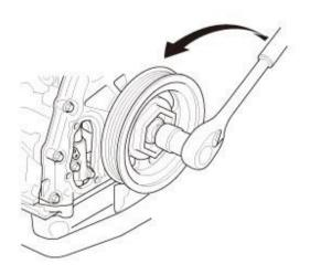
$1. \quad \text{Turn the crankshaft counterclockwise to compress the camchain autotensioner.}$
