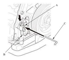
2. Rotate the crankshaft counterclockwise to align the holeson the lock (A) and the cam chain auto-tensioner (B), then insert a  $1.2 \, \text{mm}$  (3/64 in) diameter pin (C) into the holes.
