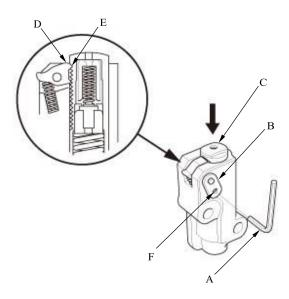
1. Compress the cam chain auto-tensioner when replacing thecam chain. Remove the pin (A) from the cam chain auto-tensioner that was installed during removal. Turn the plate (B) counterclockwise, to release the lock, then press the rod (C), and set the first cam (D) to the first edge of the rack (E). Insert the 1.2 mm (3/64 in) diameter pin back into the holes (F).
