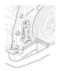
3. Remove the pin from the cam chain auto-tensioner.
