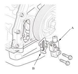
3. Remove the cam chain auto-tensioner (A) and the camchain auto-tensioner filter (B).
